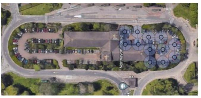
Figure 1: Estimated GSHP boreholes for Northavon House
