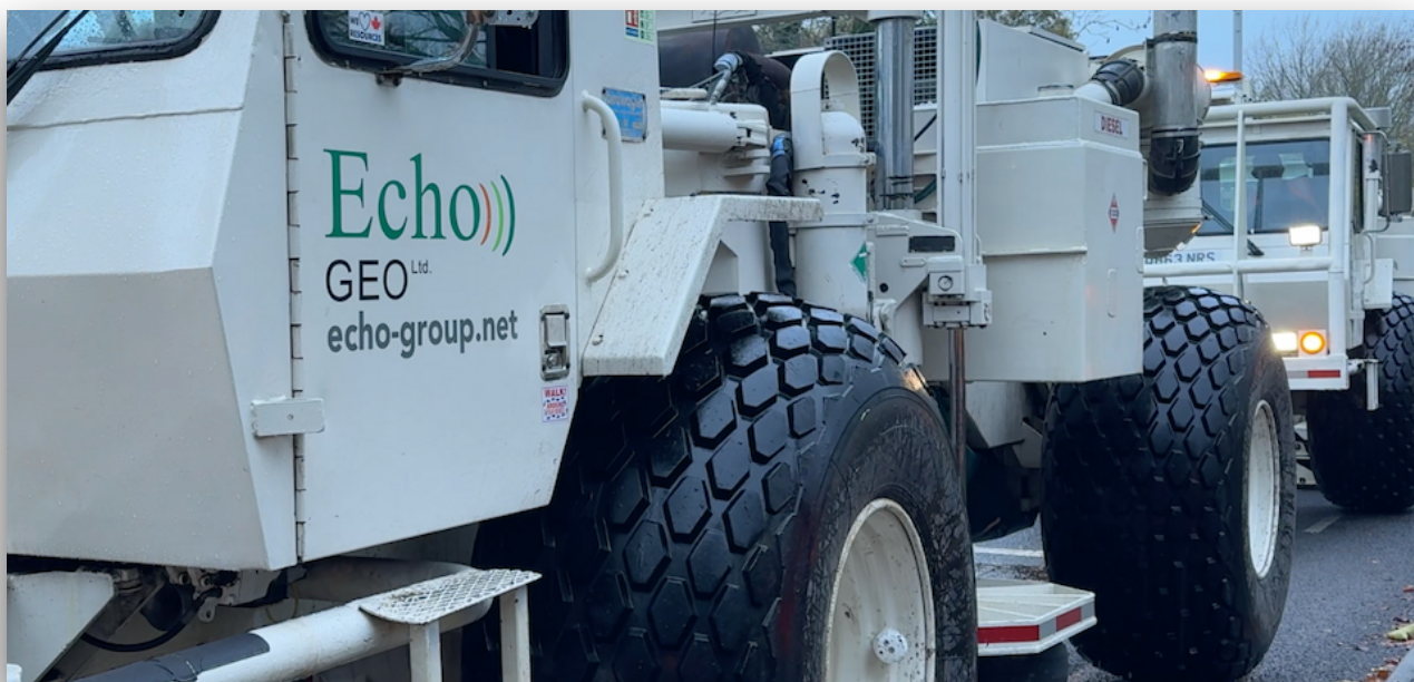
Seismic trucks in use in York checking ground conditions as part of a Public Sector Decarbonisation Scheme geothermal project at the University of York.
